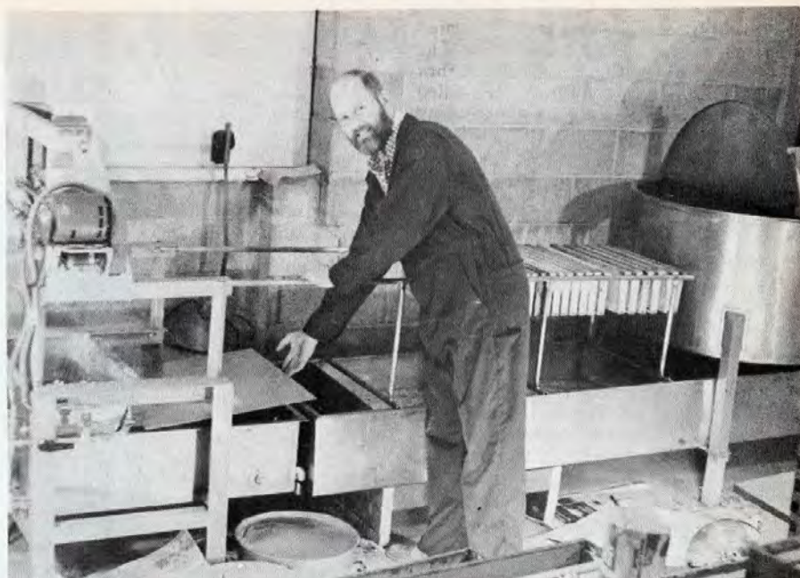
A perspective of the compactness of the basic extracting equipment. A cover is being placed over the coils of the capping melter to increase its efficiency. A pan of wax has just been drawn from the melter, showing the location of the wax outlet.
