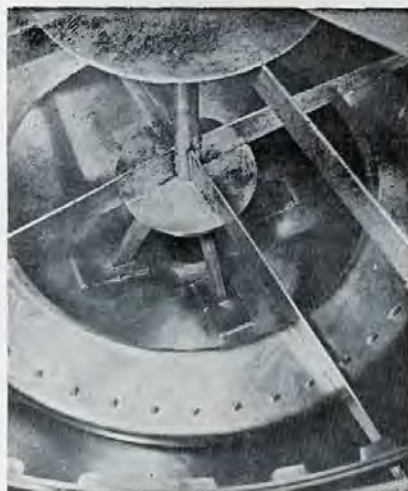
All the extractors have V-shaped sloping bottoms with large center drains. The extractor tank and reel are made of heavy 16-gauge 304 quality stainless steel. Note the continuous weld and reinforced construction on reel and tank.
