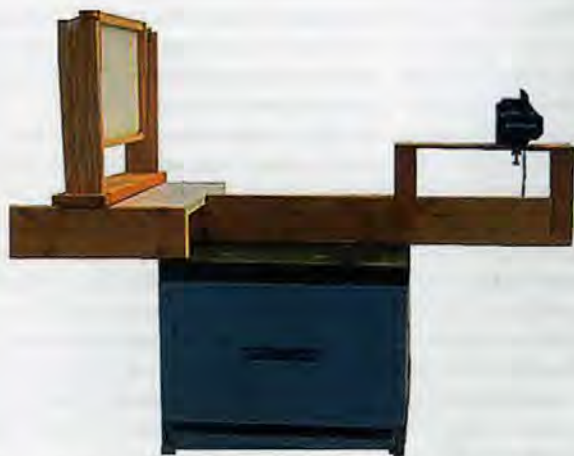
Stand for holding the digital camera and hive frame, placed on top of a super.
