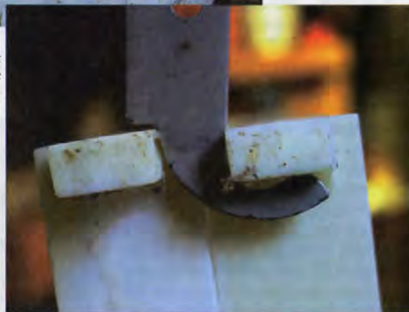
The correct placement of the hook on the Maxant hive tool.
