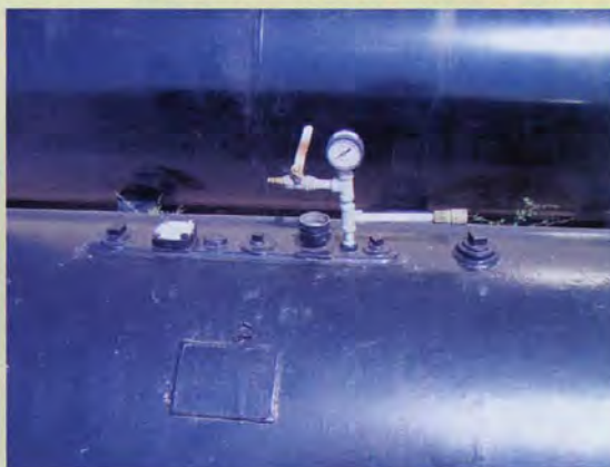
The air-loading system. The field shut-off to the feeder tank is easy to use.
