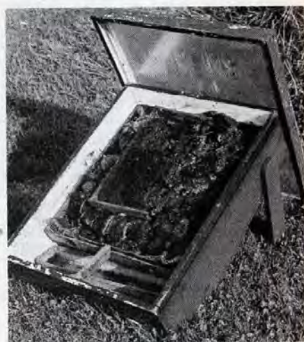
An Anderson-Penn State, homemade solar wax extractor with the top temporarily removed. For best results the inside of the extractor is painted white and the outside, black.
