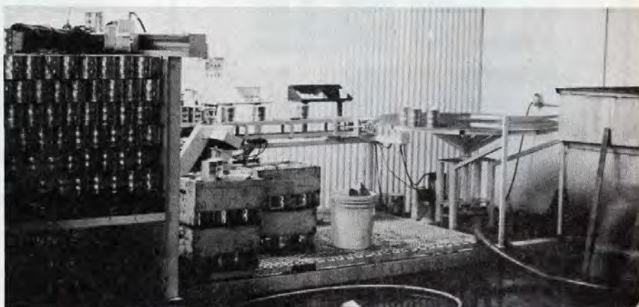
Feeder cans to accompany package bees are filled with the correct amount of syrup on this conveyor at C.F. Koehn & Sons.
