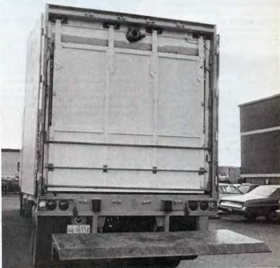
Rear end view of the unit, with inner gas-tight door closed. One of the exhaust valves can be seen above the door.
