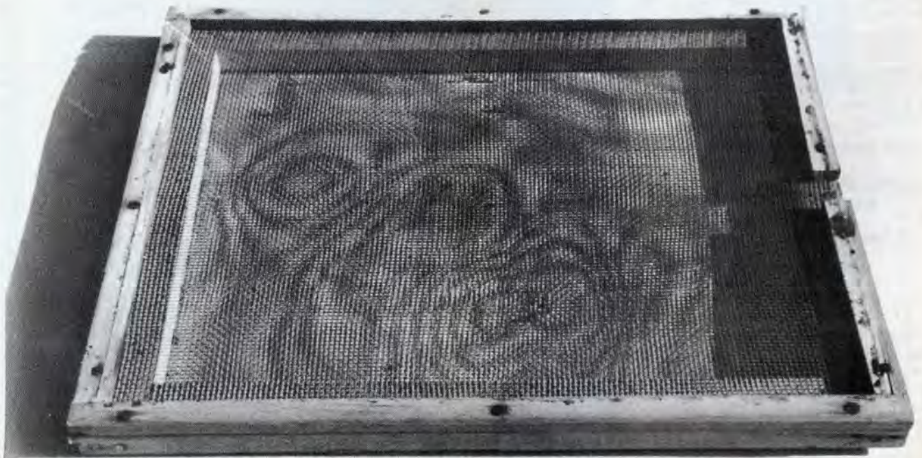
Figure 1. Double screen made with 1/8" hardware cloth.
