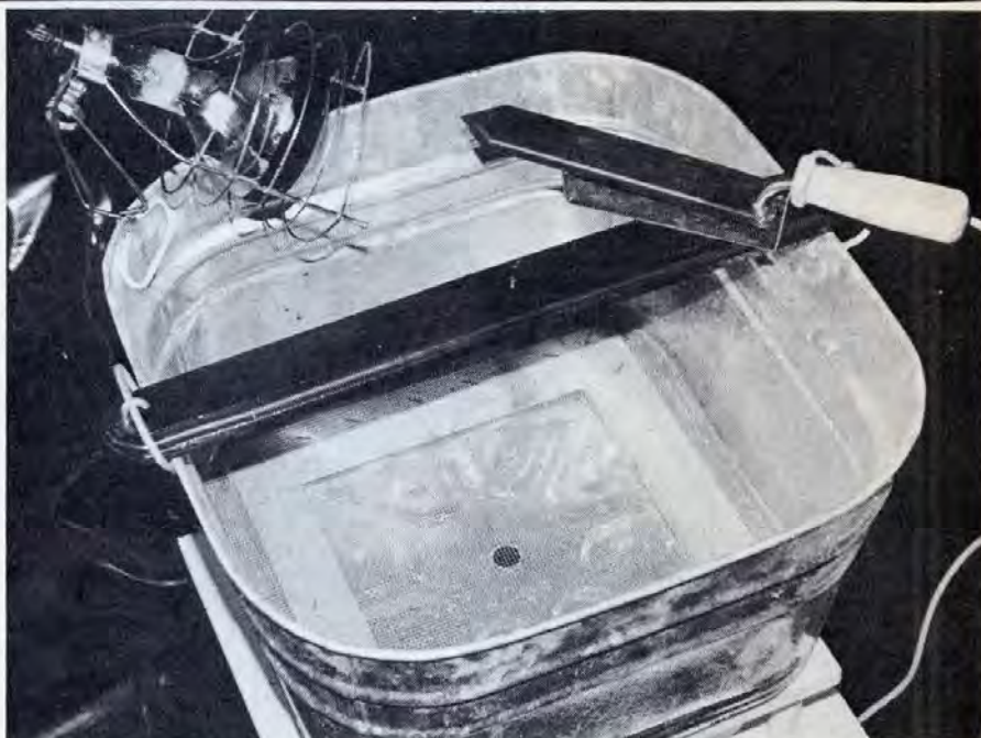
The uncapping tub from above showing the crossbar with the uncapping knife in place, the heat lamp directed to where the cappings will accumulate, the screen on its frame in the bottom, and the drain hole to direct the honey to the pan below. (Figure 2)
