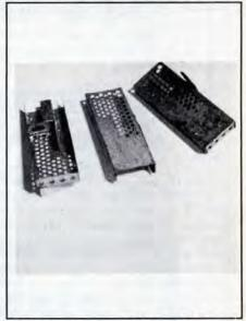
"Ideal" Chantry principle Queen releasing cage. Disassembled on left. Assembled on right.
