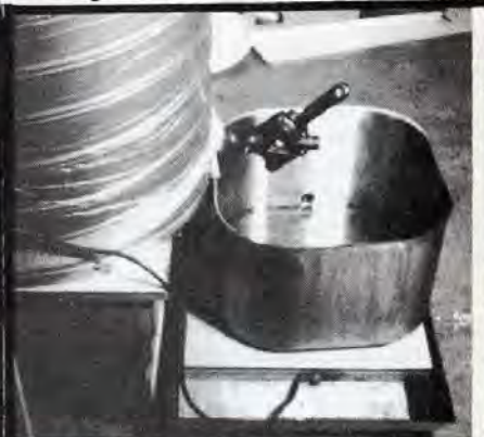
3. Honey warmer in operation. The pilot light just to right of power cord is on. Honey falling from extractor honey gate forms reflecting surface which makes it look like there are two gates in the pan. Sorry about that.
