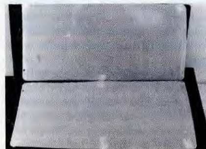
The $25 (postpaid) British-made Herring SP78 wax press for producing foundation at home.
