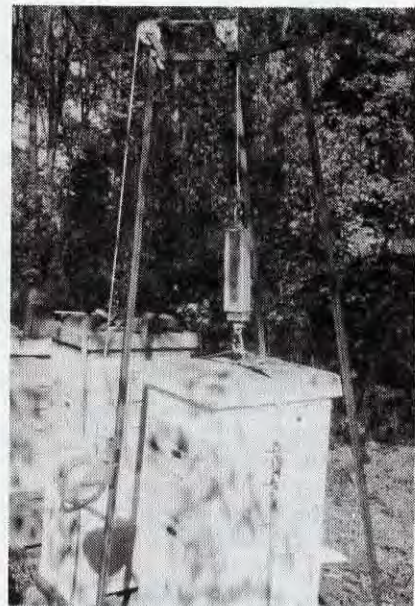
Photograph of the portable lift and scale for weighing hives.
