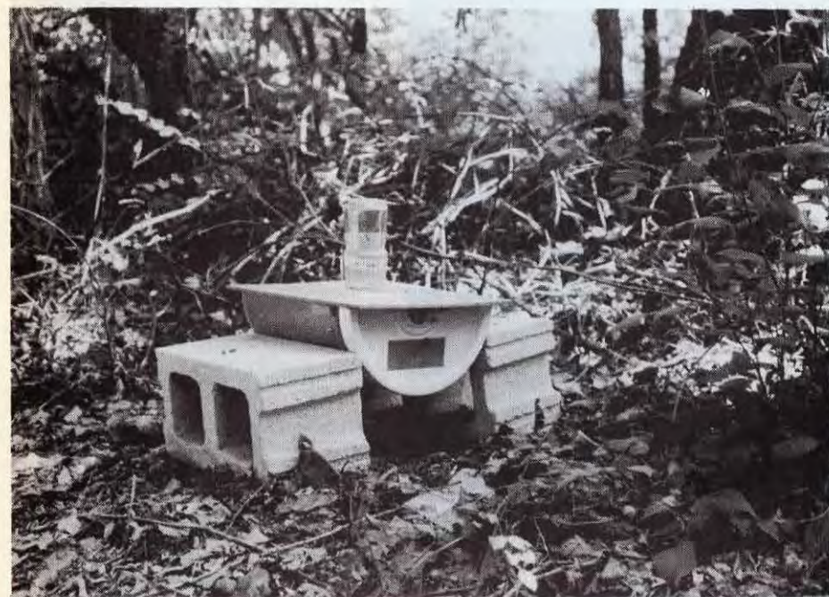
Figure 5 — Assembled unit with feeder jar in place and the whole unit supported by concrete blocks.
