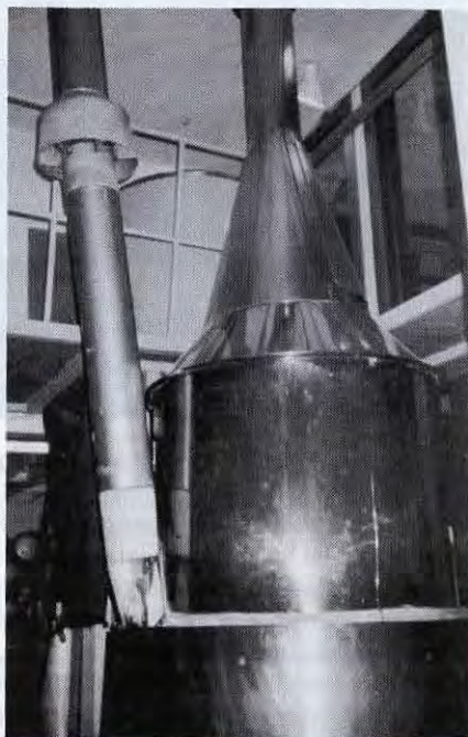
Brewing kettle where the mixture of honey, water and hops is boiled. Capacity is 387 gallons.
