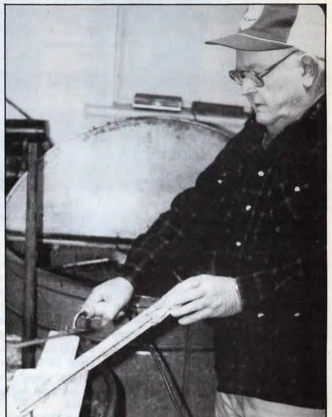
Carl demonstrates how an uncapping knife is used. Behind him is the 50 frame radial extractor used in his honey operation.
