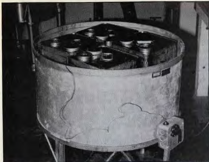
Tank (water bath) for heating 5-gallon cans of honey. The sensing element, at end of the long wire, is in the water, not the honey.
