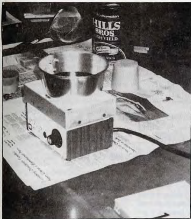
Once your dark and dirty wax is melted, keep enough heat on so it remains liquid, but not so much to cause it to boil.
