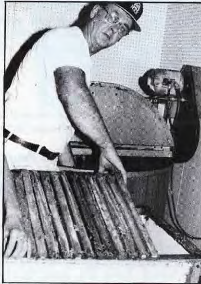
Uncapped and cleaned frames are put in the extractor that isn't running. "You can't believe how much cleaner our honey is because we uncap well, and then remove all the stuff off the top," says Dorothy. The Tonn's have two extractors, which they operate in rotation. Identical, they each hold 55 Illinois depth frames, have variable speed control and do everything we need. "Having two machines is good because there's no lag, and if one's down, you're not out of business until it gets fixed," says Tom.
