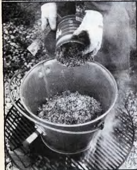
This is the pail mentioned in the article. A hole has been made in the side about three quarters of the way up and a pipe nipple inserted and fastened (welded). A "V" shaped baffle could be added to the inside to make this even more efficient. Put about an inch of water in the pail, then add the cappings.
