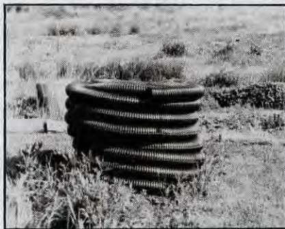
Drainage is an often overlooked problem. Heavy, wet soils do not support many legumes. Plastic drainage pipe can be the answer.
