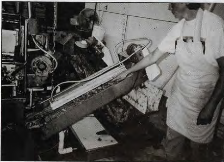
An infrared light heats the wax to the melting point. The chain conveyor takes the wax to the compression chamber.
