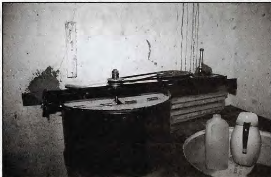
Senor Alonso's homemade 16-frame radial extractor.
