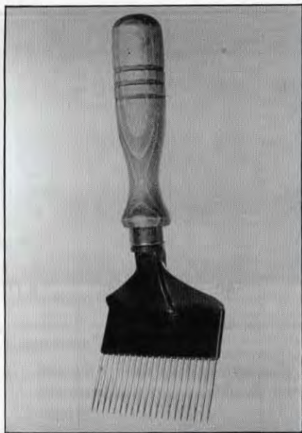
A Cappings Scratcher, used to get at areas missed by conventional knives. Always good to have around.
