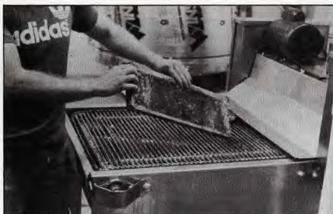
The undamaged and uncapped frame exits the machine ready for the extractor.
