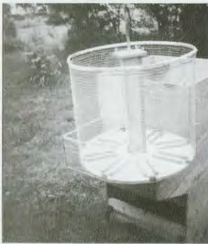
Detail of basket showing bottom supports and spindle top.
