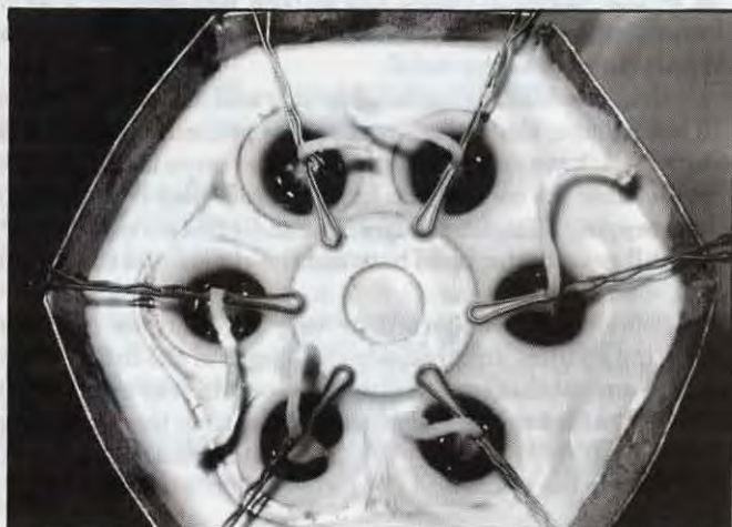
After the pour. The wax has started to set and contract. It will be ready for topping off very soon. Note that there is some wax in the base already.
