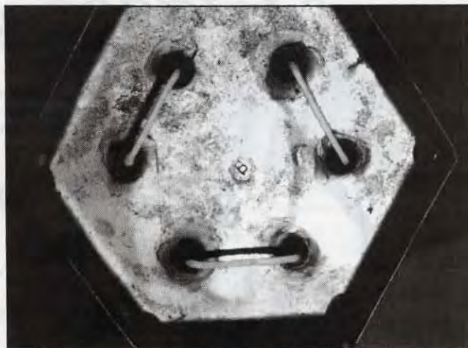
Base of the mold. Each length of wicking is long enough to string through two adjacent candles. They are held taut by mild tension from the bobby pins at the other end of the mold.
