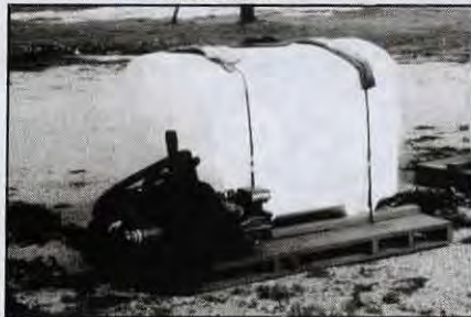
A 240 gallon feeder tank, with pump and hose.
