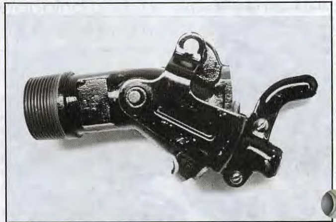
Don't forget the little things, like cleaning out gates and valves. Dirty gates will be frozen solid by next summer. Hot soapy water works best.
