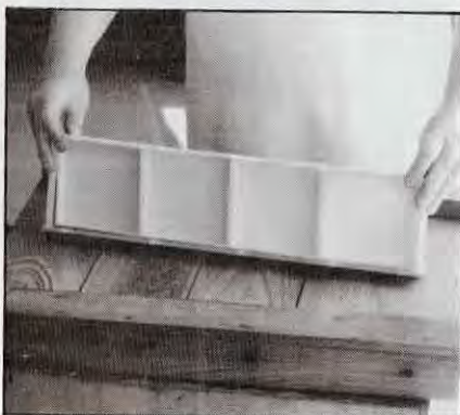
When inserted correctly the sections will close exactly, with no gaps or holes. This is critical for good comb foundation.
