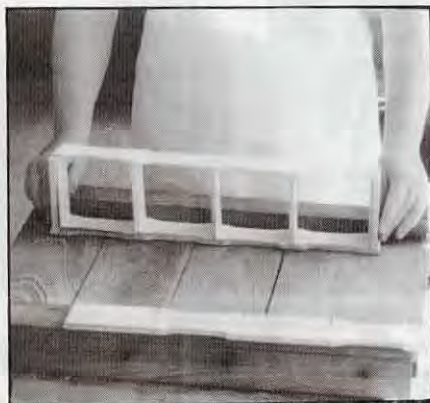
When setting the boxes in the holder, make sure none of the splits are on the bottom.
