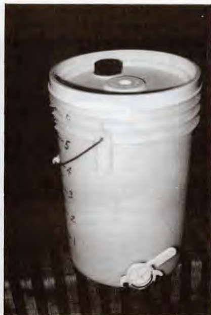
A six gallon pail with a 1-1/4" honey gate makes a good settling and bottling tank.
