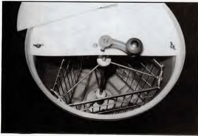
This tangential style extractor will hold either three deep or six shallow frames. The crank on top can be removed and replaced by a variable speed drill.
