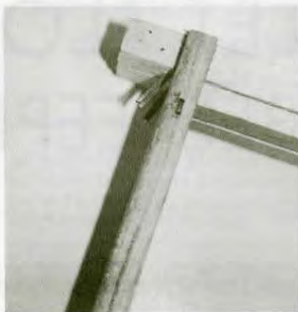
Things that can go wrong – the staple from the top bar misses the end bar. If your thumb is in the vicinity life gets interesting, and usually painful.
