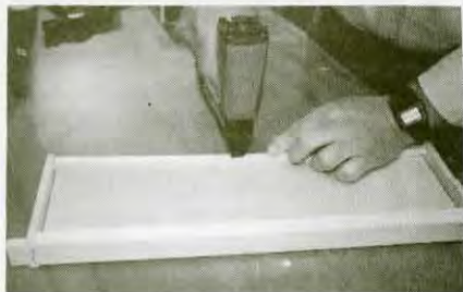
A finishing touch is fastening the two-piece bottom bar and foundation sheet snugly.
