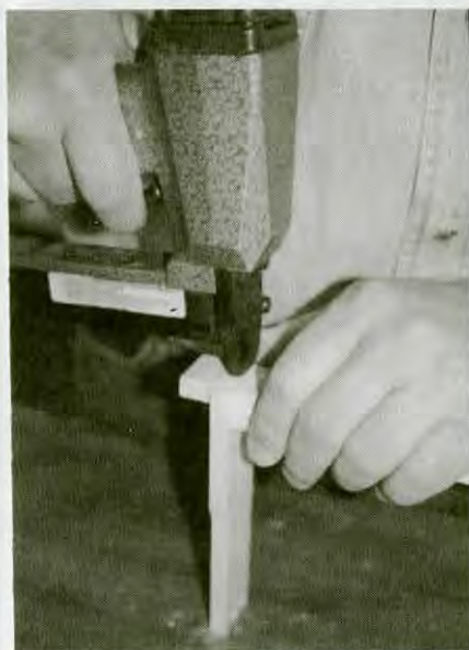
Drive 2 staples from the top down into the end bar.
