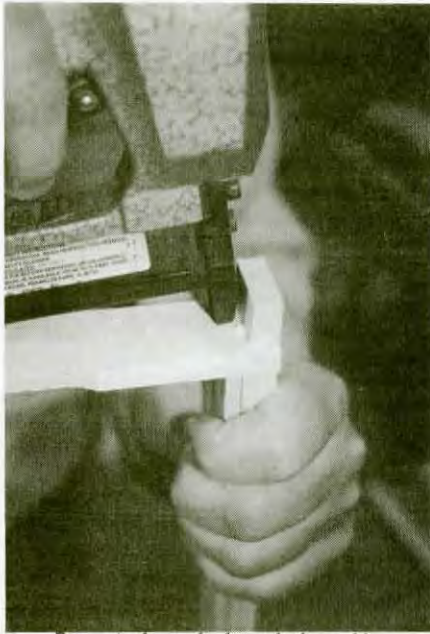
Put a single staple through the end bar, horizontally into the top bar.
