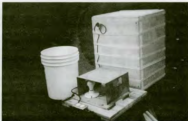
Constructed heater, showing box in back, wrapped in tape, stand in front, with bulbs in place, and outlet.
