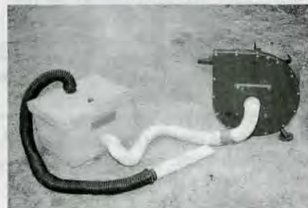
The unit, including box, hoses, nozzle and blower. The white hose is connected to the intake opening of the blower using a piece of plywood. On the left, the standard package that sits inside is shown. Air flow goes from the nozzle, through the black hose, into and through the box, continues through the white hose and into the blower.
