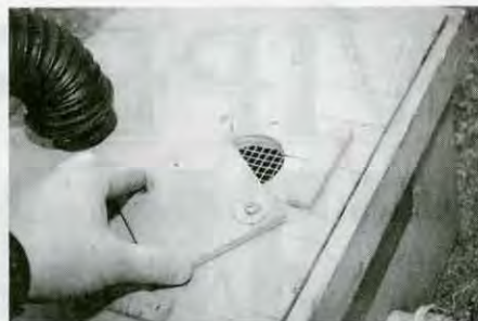
The vacuum pressure shunt, or pressure regulator, hinges on top, and controls the airflow inside.
