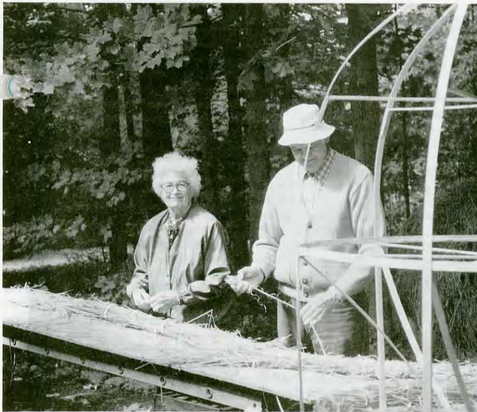
Frances Alloway and Dick Miller form the rye-straw rope which was used to build the skep.
