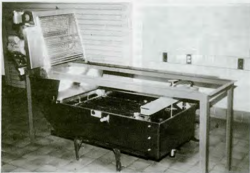
A Cowen unit uses knives to remove the cappings. Partially and fully automatic models are available.
