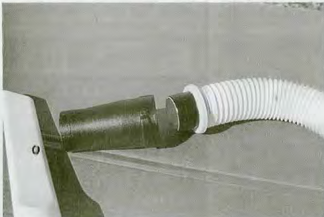
Cut off air outlet tube with taped hose coupling.
