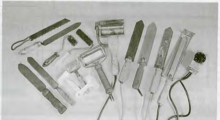
A collection of hand-held uncapping devices. Pictured, from L to R: cold knives (4); Hackler Punches (2), scratchers (3), planes (2), electric knives (3).
