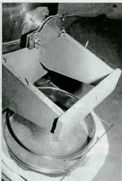
Liquid honey runs out of the gate. It can be first-strained by having a cloth filter stretched over the wood frame, and then second filtered below.
