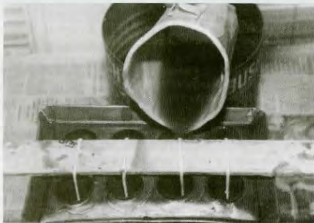
Carefully pour the clean wax into the mold cavities using a small cup or ladle.
