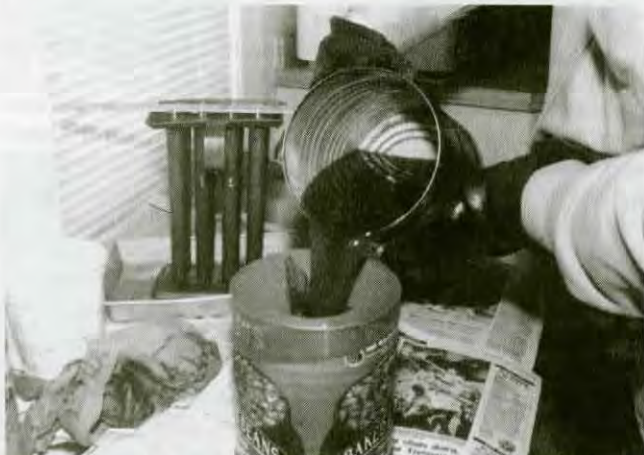
Carefully pour the hot wax through the strainer into the tin can. Repeat two or more times to ensure that as many impurities as possible are removed from the wax.
