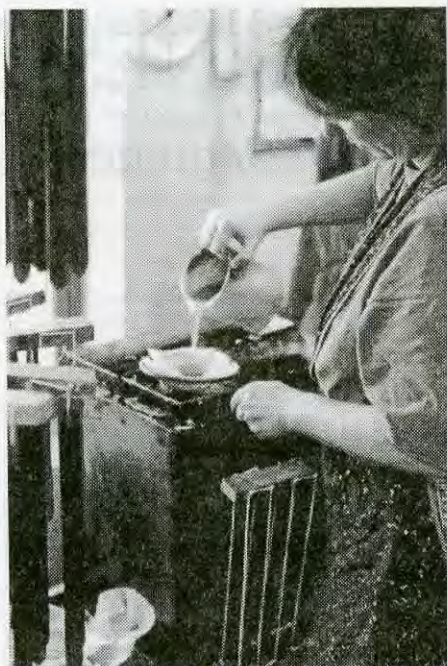
Sharon straining wax dipped from the back section of the tank into the front section through a Bounty™ paper towel.
