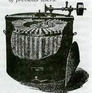
Left, a 1922 Buckeye full speed reversing extractor, 4 frame. Right, an 8 frame Buckeye
