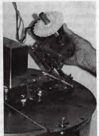
Bob purchased a variable speed, reversible motor from a local hardware store. He mounted the motor on a hinge because there was no clutch system. When disengaging the motor he lifts the motor so the gears no longer are in contact. The extractor spins much longer than the motor, so if left engaged the motor would burn out. Because it is reversible, he can reverse the motor to spin frames in the opposite direction, completely emptying cells of honey.
