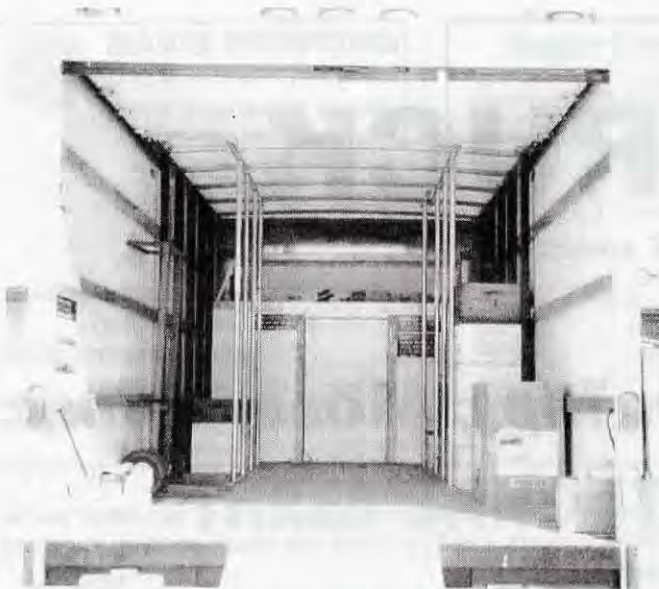
Inside, ceiling to floor poles and on-the-floor braces keep supers from moving. Storage space in the 'attic' works for small items, and a walkway in the center makes it all easy to get to. Tall enough to prevent bendings, it also saves the back when working inside, and everything is high, dry and clean.
