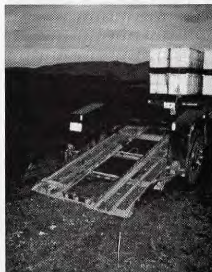
The forklift trailer, made sturdy. When the machine is unloaded the bed tips down. When loaded, the bed tips up to be level. The machine is chained on in two places.
