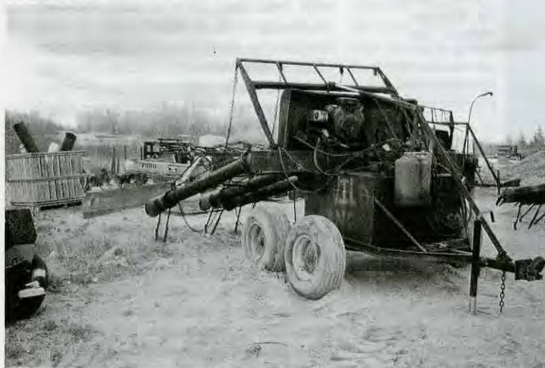
The old flame thrower, used to burn off plants. It is seldom used now.
