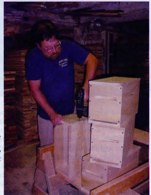
Assembly. Screws make repairs easier, but make sure you don't split the ends.
