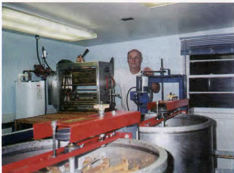
Bob Hughes at his Silver Queen uncapper. Note the hot water tank (white) to the left. This provides hot water for the knives.
