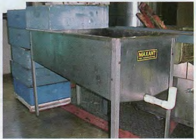
An uncapped frame tank. It can also be used as an uncapping tank.
