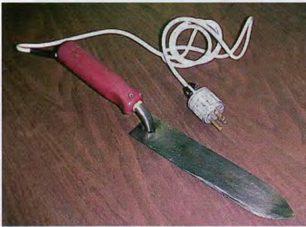
An electrically-heated uncapping knife.
