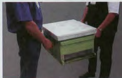
A lightweight hive carrier made from 1" steel tubing.
