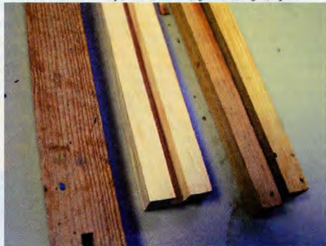
Bottom bars. Left, solid; center, grooved; right, split.
