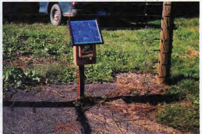
A solar charger. The bigger the fence, the bigger charger you will need.
