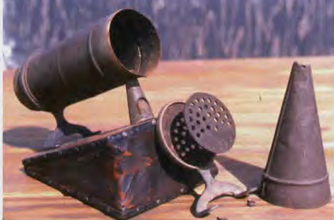
Figure 6: A Quinby smoker disassembled for cleaning. Now it's easy to scrape out the soot from the tube. Cleaning the grate is also easy, and now it's even easy to clean under it. All that seemingly odd construction had a definite purpose and was actually quite clever. It just wasn't apparent since such smoker disassembly is unheard of today. Also note the opening in the pipe connecting the bellows and firebox to let in air between bouts of smoking the bees.
