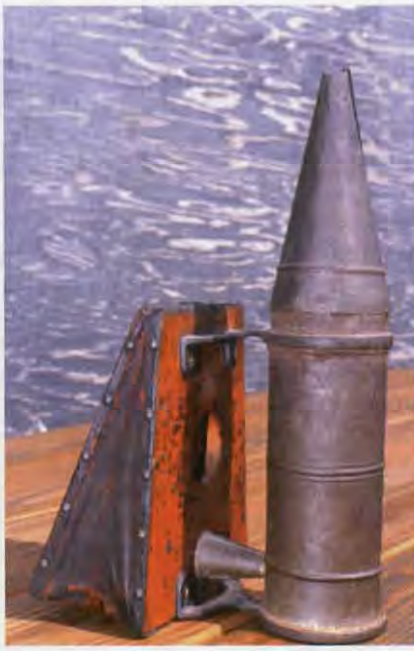
Figure 3: A Quinby smoker as sold by L.C. Root. Note the cast iron brackets attaching the bellows to the firebox. Also the lower bracket and the bottom of the smoker are made of one piece of iron. Why this odd construction?
