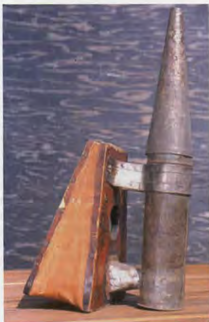
Figure 2: An early Quinby smoker. The smoker has a solid pipe connection between the bellows and firebox. The round hole in the bellows, covered internally by a piece of tin, is a one-way air valve.
