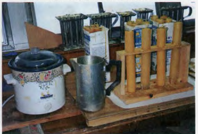
Equipment used to pour candles includes a crock pot, pouring pitcher and polyurethane and metal molds.
