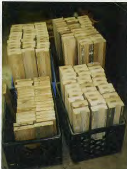
Frame parts ready for assembly. Photo 2.
