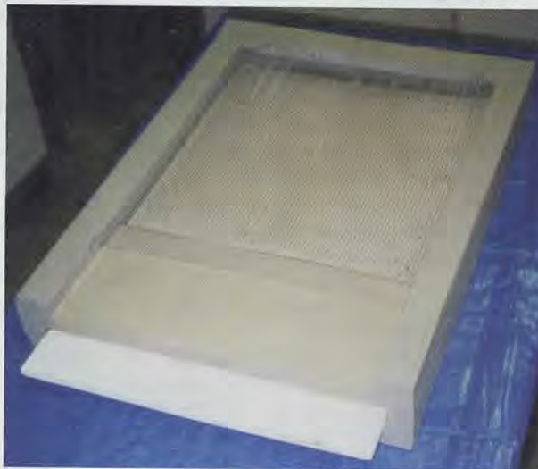
Finished screened bottom board.
