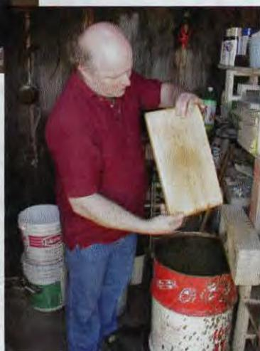
*Joe examines the blank as he prepares to dip it into the water tank. Water ensures the wax will peel off cleanly, and the blank is dipped into water before each new sheet is made.*
