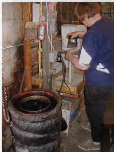
*Before beginning work for the day, Dee sands all surfaces of the wooden dipping blank to ensure water will adhere to it. When dipping, the wax sheets peel off the easily if the wood is wet. Wax for foundation making is melted in the dipping tank (left foreground). The tank is insulated, water jacketed, electrically heated, and thermostatically controlled.*
