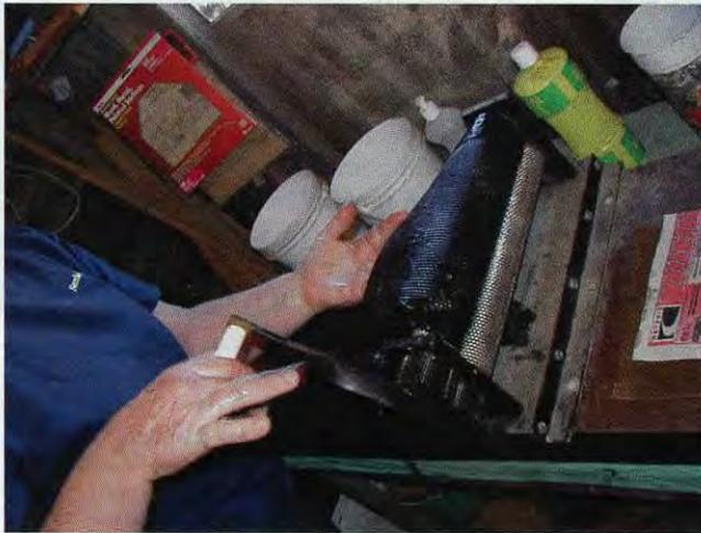
The wax, enclosed in the thin plastic is then rolled through the mill. These hand-cranked rollers are specially made by Tom Industries of Yuma to produce a cell that measures just under 4.9 mm. Joe and I later met Tom on our way west, and saw his shop. The newspaper pieces shown are used to separate the fresh sheets of foundation to prevent their sticking together.
