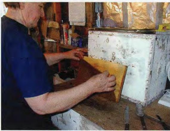
While still soft, two blank sheets of wax are peeled off the damp board - one from the front and one from the back —and stacked awaiting milling. Scraps go back into the melting tank.
