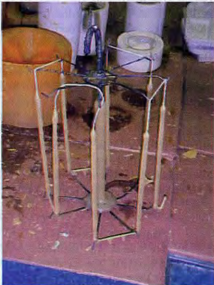
A shop built jig for dipping eight candles at once.
