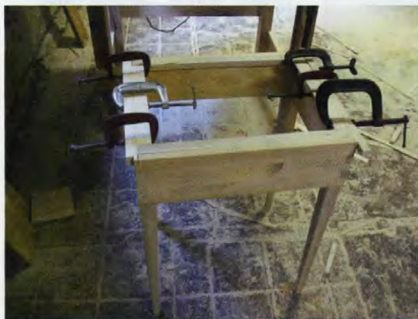
Attaching braces to the apron.
