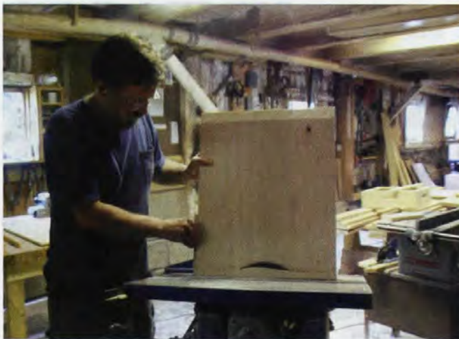
Beveling underside of tabletop.
